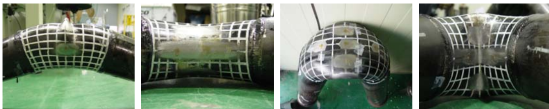
(a) Failure modes according to the thinning location and the bending direction
